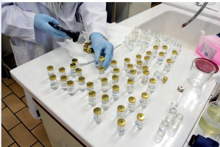
Preparation of volatile chlorinated samples
