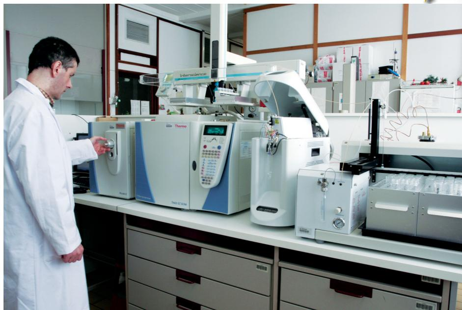
*Analysis of aliphatic and aromatic hydrocarbons (VOCs) and chloral hydrates by Purge and Tap coupled with a GC-MS Ion Tap*
