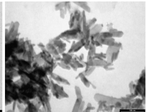
Copper oxide (rod-shaped)
