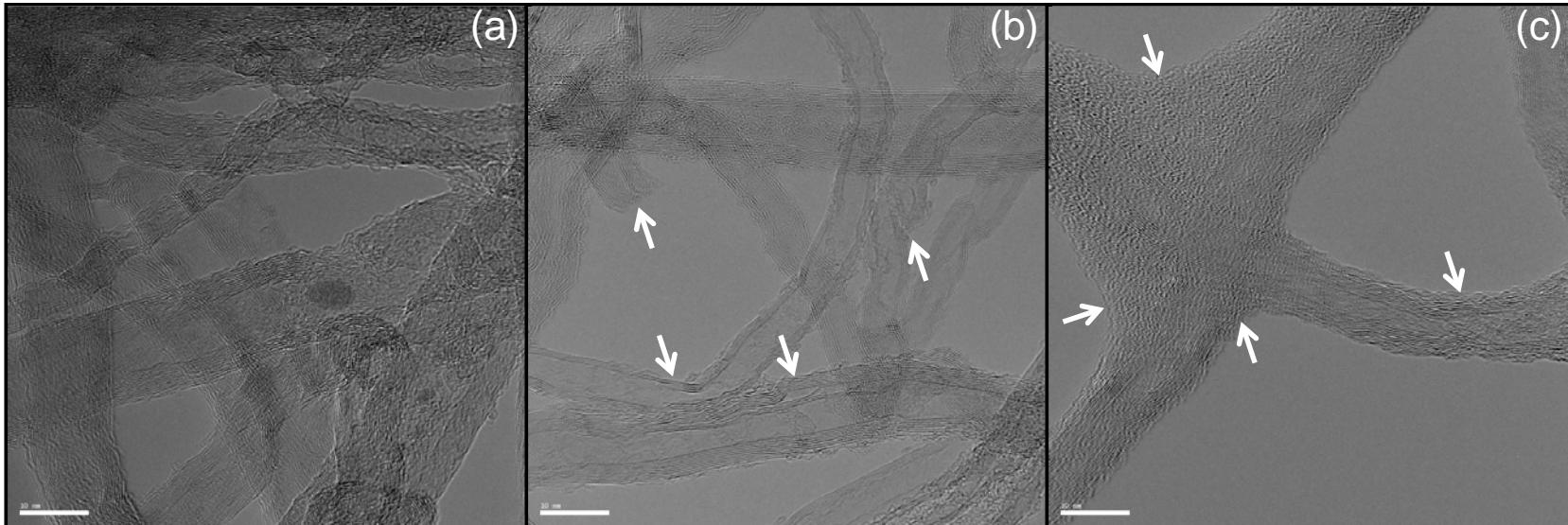
Sonication induces degradation (even breaking) in MWCNT outermost wall
