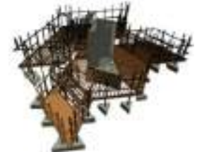
4. 2 by 6" red cedar posts & beams
