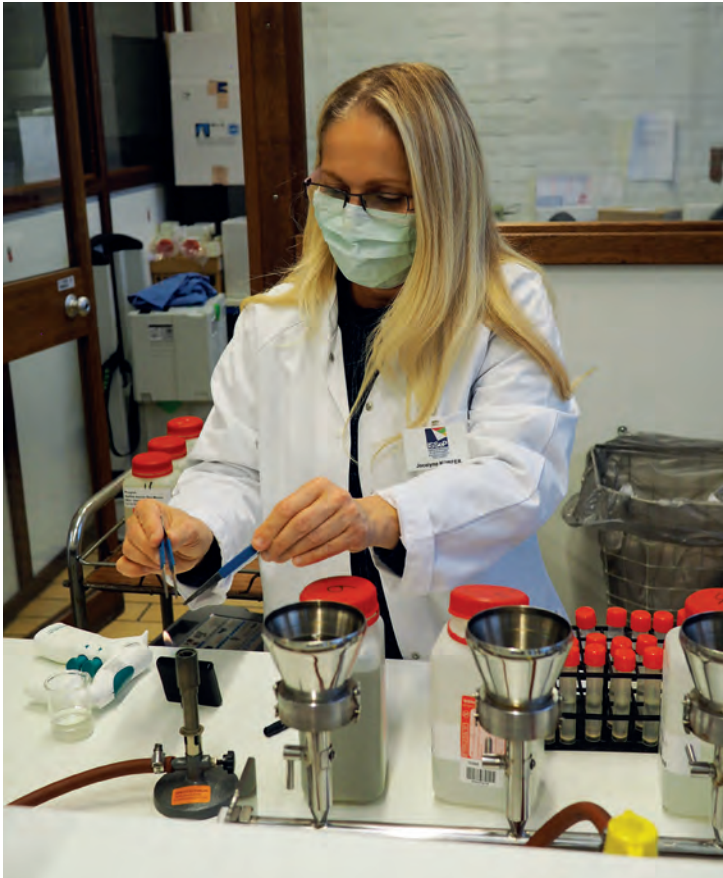
Microbiology cell. Filtration of cooling tower samples: search for legionellae
