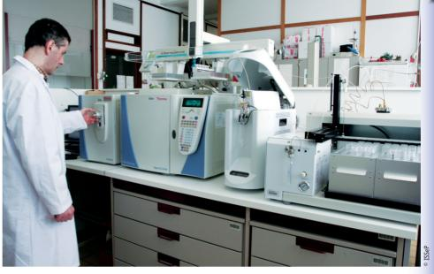
Analysis of aliphatic and aromatic hydrocarbons (VOCs) and chloral hydrates by Purge and Tap coupled with a GC-MS Ion Tap
