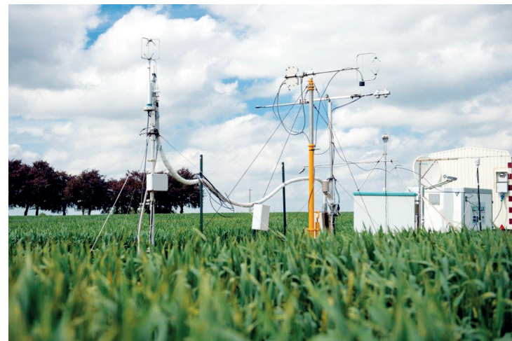
Measurement of greenhouse gases flux from agricultural crop (ICOS, Integrated Carbon Observation System)
