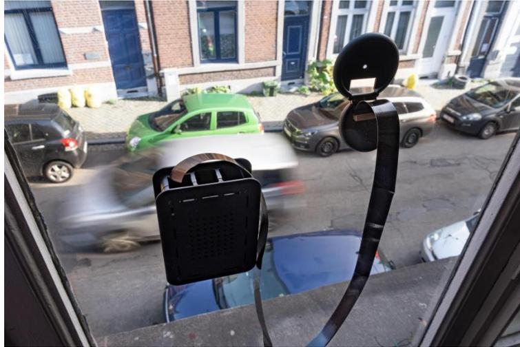
**FIGURE 6. DISPOSITIF TELRAAM (MICRO-ORDINATEUR RASPBERRY PI ET CAMÉRA) POUR LE COMPTAGE DU TRAFIC.**
