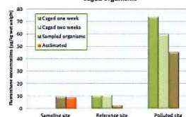
Fluoranthene concentrations in organisms from sampling site, reference site, polluted site and caged organisms
