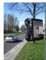
Figure 10 - Radar for automatic traffic count. Distinction is made between short and long vehicles.
