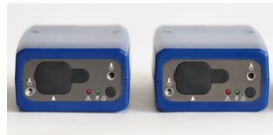
Figure 3 - AE51 portable aethalometers working at 880 nm. Dimensions: 117 mm x 66 mm x 38 mm. Weight: 280 g.
